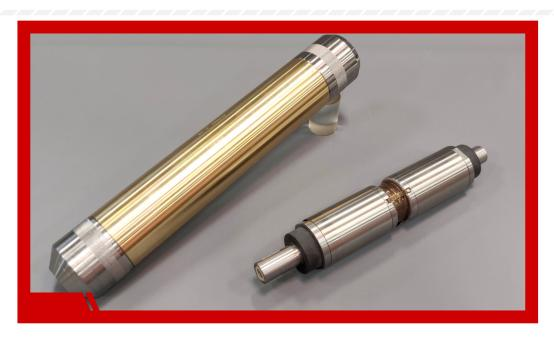
Collar Locators are based on the principle that changing magnetic flux within the instruments sensor coil generates voltage across the terminals of that sensor coil. The magnetic field of a CCL magnet is affected by any magnetically sensitive material, such as tubing. A collar or joint in the tubing changes the magnetic flux field including the flux passing through the sensor coil ends adjacent to the magnets, causing a signal to be generated at surface.
